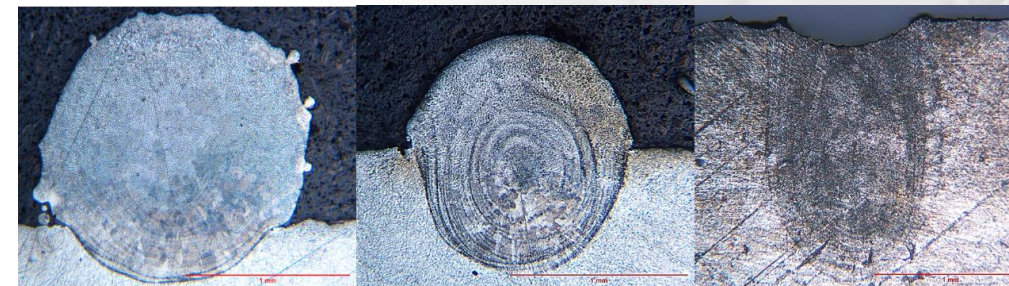
(a) Conduction (b) Transition (c) Keyhole Example cross-sections of single tracks, illustrating the three different regimes
