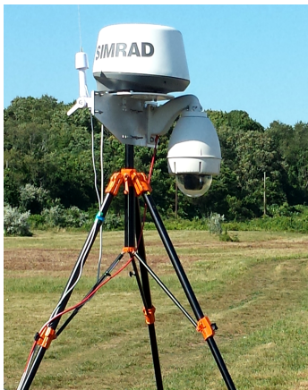
Figure 7. The land-based part of the low-cost sensor suite consisting of Radar, Camera and AIS.
