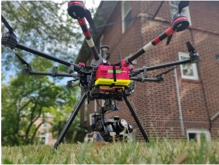
Figure 3. SDR for aerial recording of RF signals installed on a DJI S1000 UAS.
