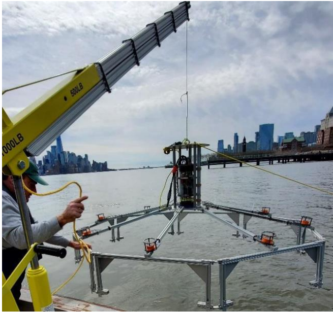
Figure 8. SPADES-2 during deployment in the Hudson River.
