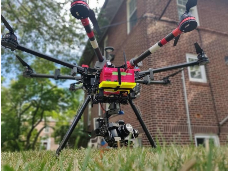
Figure 2. SDR for aerial recording of RF signals installed on a Stevens DJI S1000 drone.
