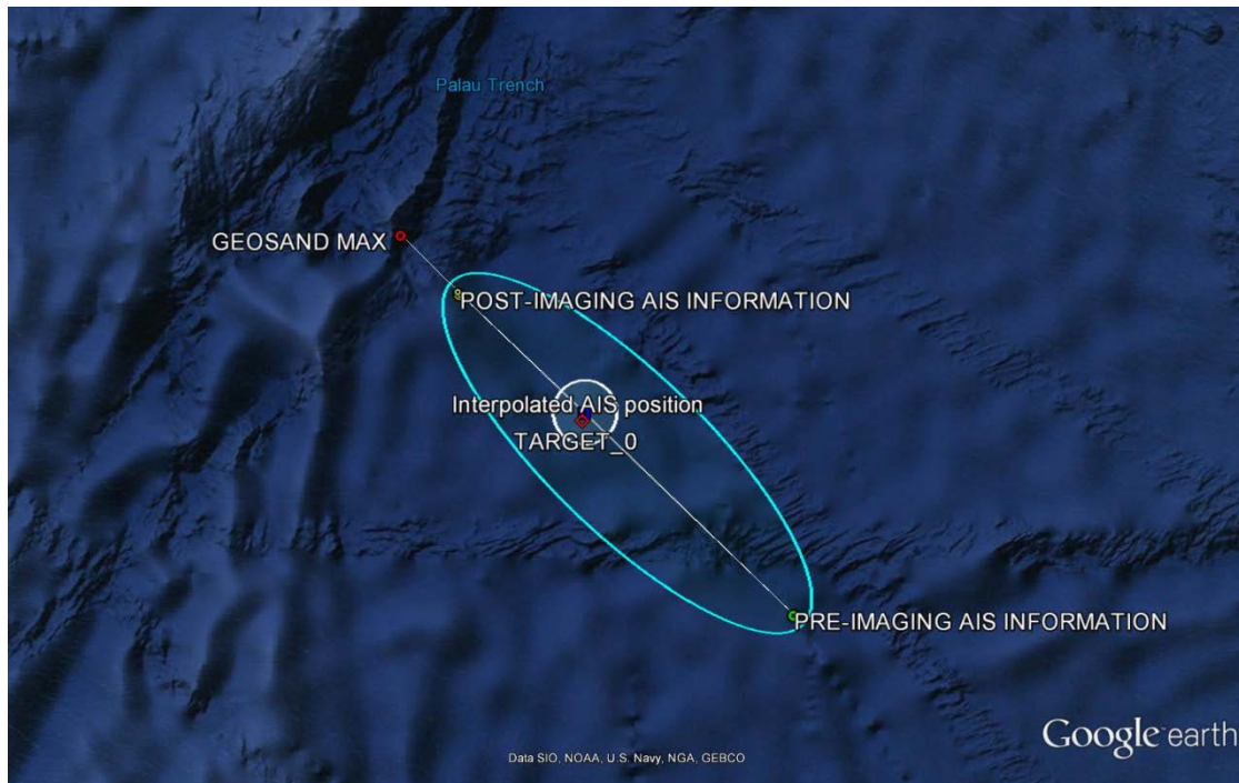
Figure 5: Uncertainty ellipse associated with a detected target in a SAR image which is a routine output product generated by CSTARS' SeaSentinel.
