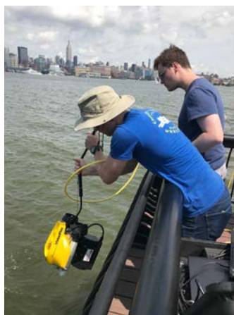
Figure 9. Doctoral Fellow, John Martin tests the odometry readings from sensors on an ROV.
