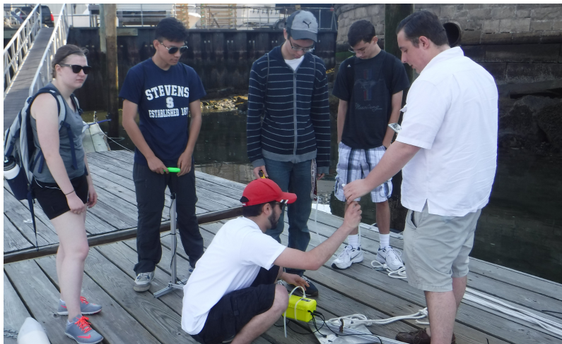
Figure 8: Students on the Buoy Noise Team prepare a passive acoustic recording system for deployment and experiments at the U.S. Merchant Marine Academy.
