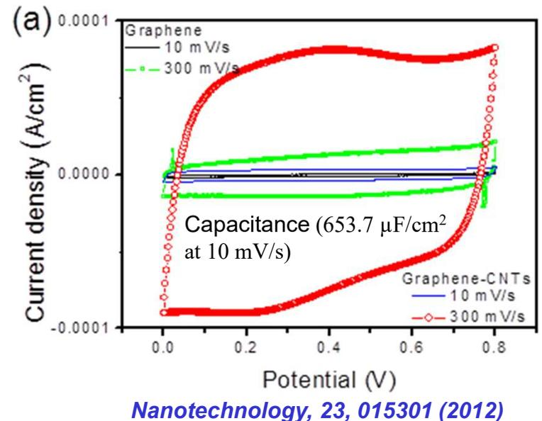
**Supercapacitor:** An electrochemical capacitor with
