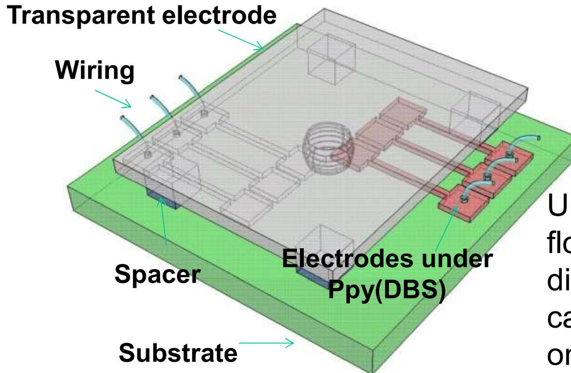
Unlike continuous-flow systems, discrete droplets can be manipulated on a substrate:
