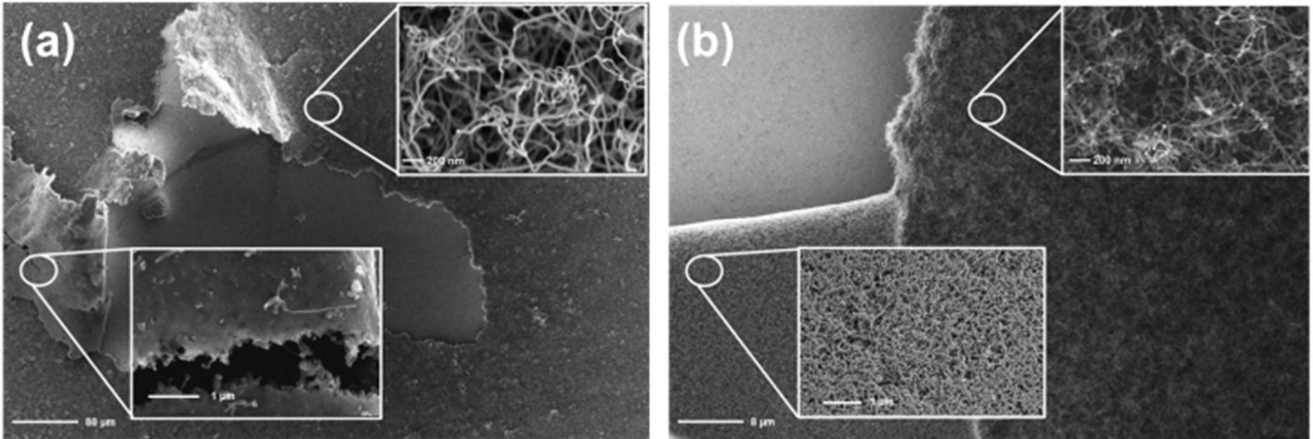
(a) intact graphene substrate and (b) without graphene (etched away)
