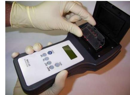
**Low-cost, hand-held device (powered by a AAA battery) containing complex liquid handling assays.**
