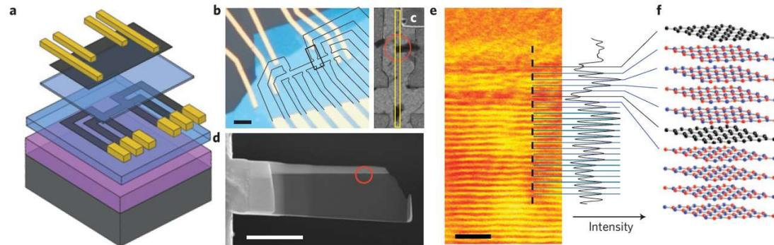
**Figure 1 | Cross-sectional TEM of graphene-hBN heterostructures. a**, Schematic of one of our devices: two graphene monolayers (dark grey) are interlaid
