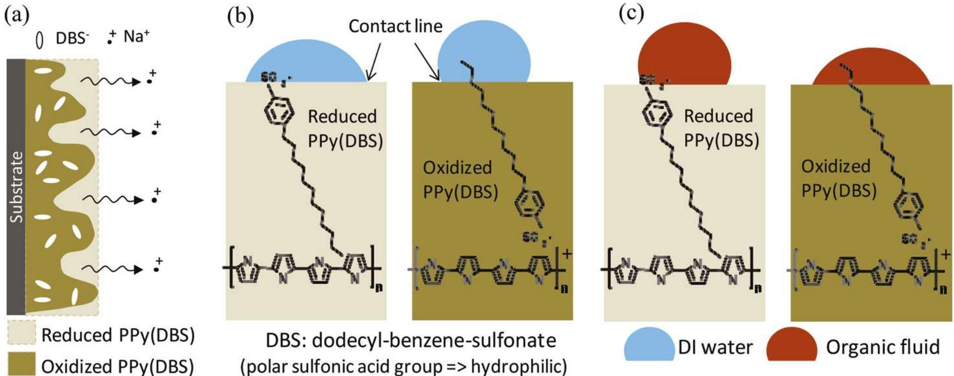
*Reduced PPy(DBS) surface exhibits higher surface energy than the oxidized case.*
