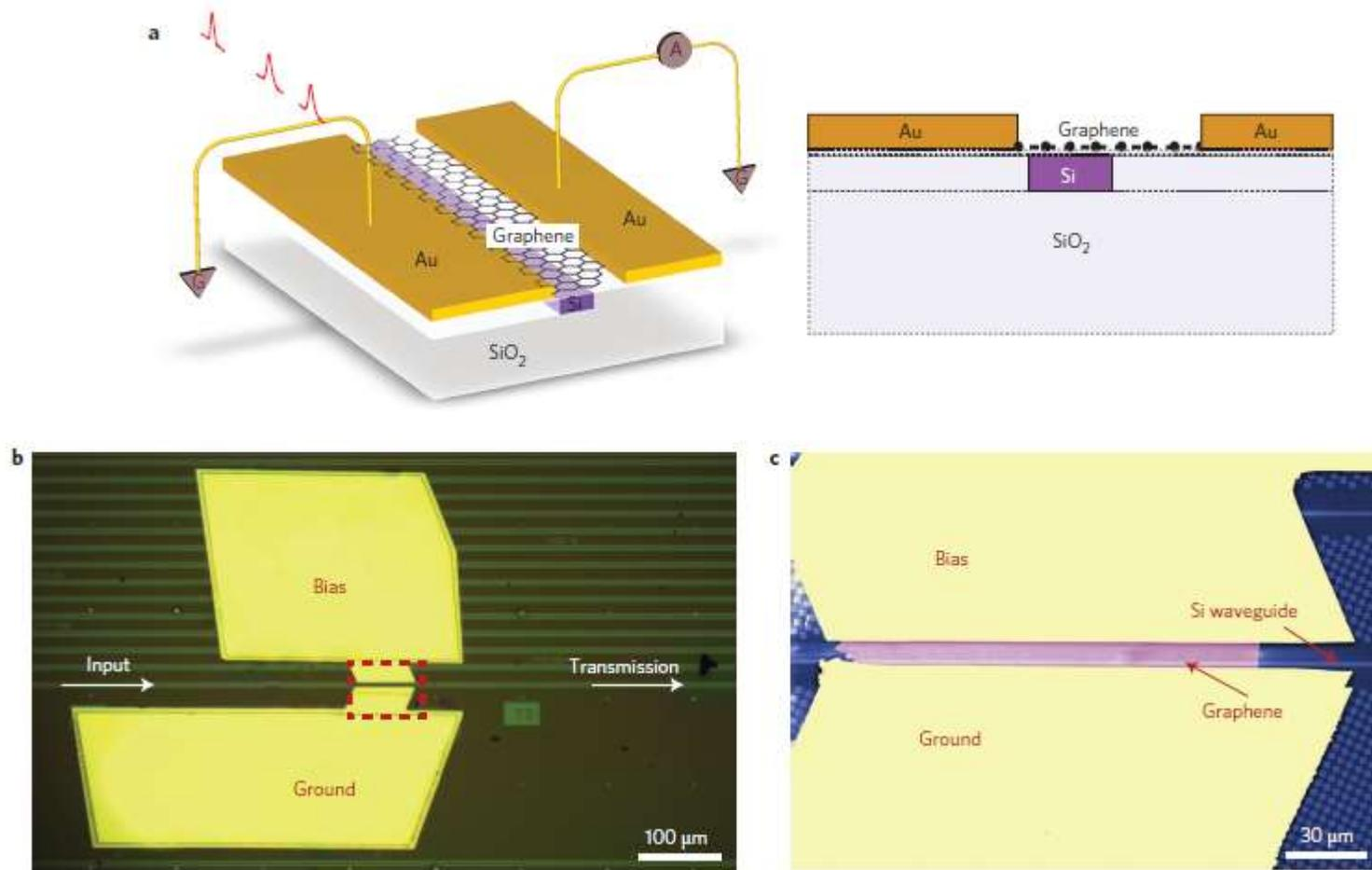
**Figure 1 | A waveguide-integrated graphene photodetector.** a, Schematic of the device. The silicon bus waveguide fabricated on an SOI wafer is planarized
