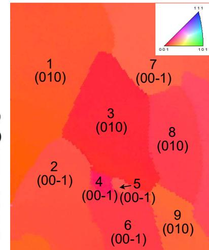
2-lobed symmetrical curvilinear graphene domains specifically on Cu{100} surface orientations; **its growth and morphology are dependent on the underlying Cu crystal structure** → *important towards tailoring graphene properties via substrate engineering*
