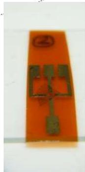
Transferred graphene on flexible substrate
