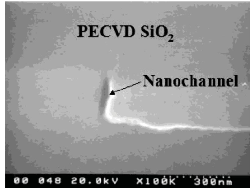
**Figure 3.** SEM micrograph of nanochannel with PECVD oxide sealing: The width is approximately 25 nm.
