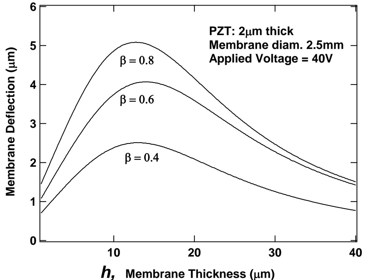
Maximum deflection occurs at intermediate membrane thickness
