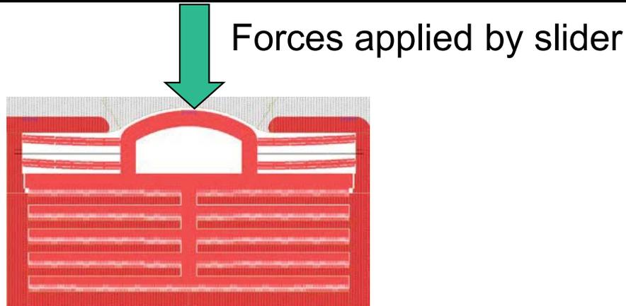
Assuming the static friction coefficient is 0.24, the estimated push force when actuating is approximately 24 mN. In power-off mode, the estimated clamping force is approximately 48 mN.
