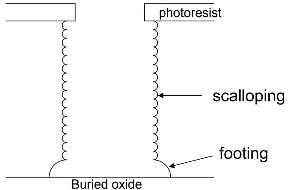
Typical surface profile of DRIE sidewall
