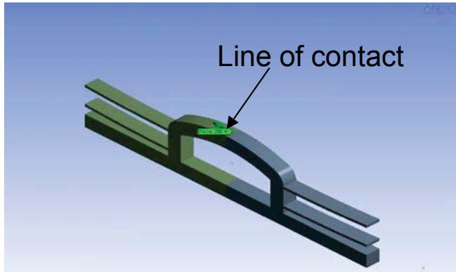
*Fixed normal displacement: 10  $\mu\text{m}$  at the line of contact*
