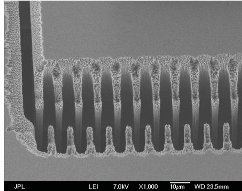
The bottom of the comb is over-etched.
