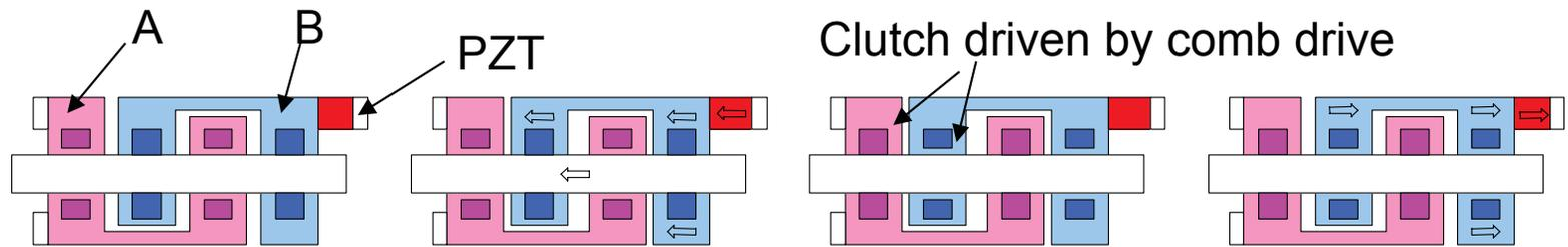
(a) Unit A released. Unit B clutched. (b) Unit B laterally moved. (c) Unit A clutched. Unit B released.
