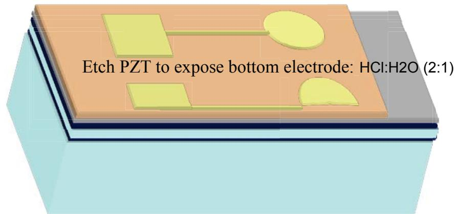
Etch PZT to expose bottom electrode: HCl:H<sub>2</sub>O (2:1)
