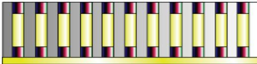
3) Nanowire / electrodeposit soft magnetic material
