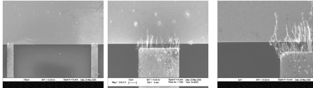
SEM images of magnetically aligned nickel nanowires on ferromagnetic electrodes.
