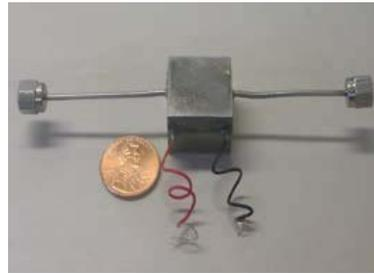
High-pressure, leak-tight microvalve for proportional flow control
