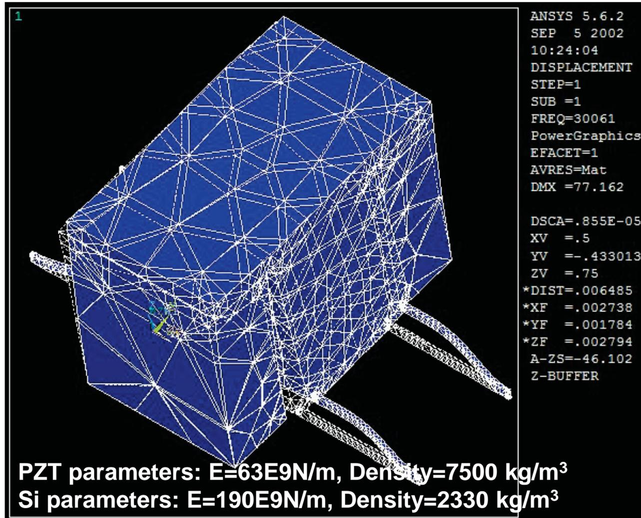
**Microvalve with PZT (1<sup>st</sup> mode,  $f_0=30\text{kHz}$ )**
