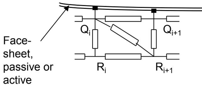
The flexures are bonded at the points  $\{Q_i\}$  and  $\{R_i\}$ , and the angles between the tangents to flexures at the points remain constant.
