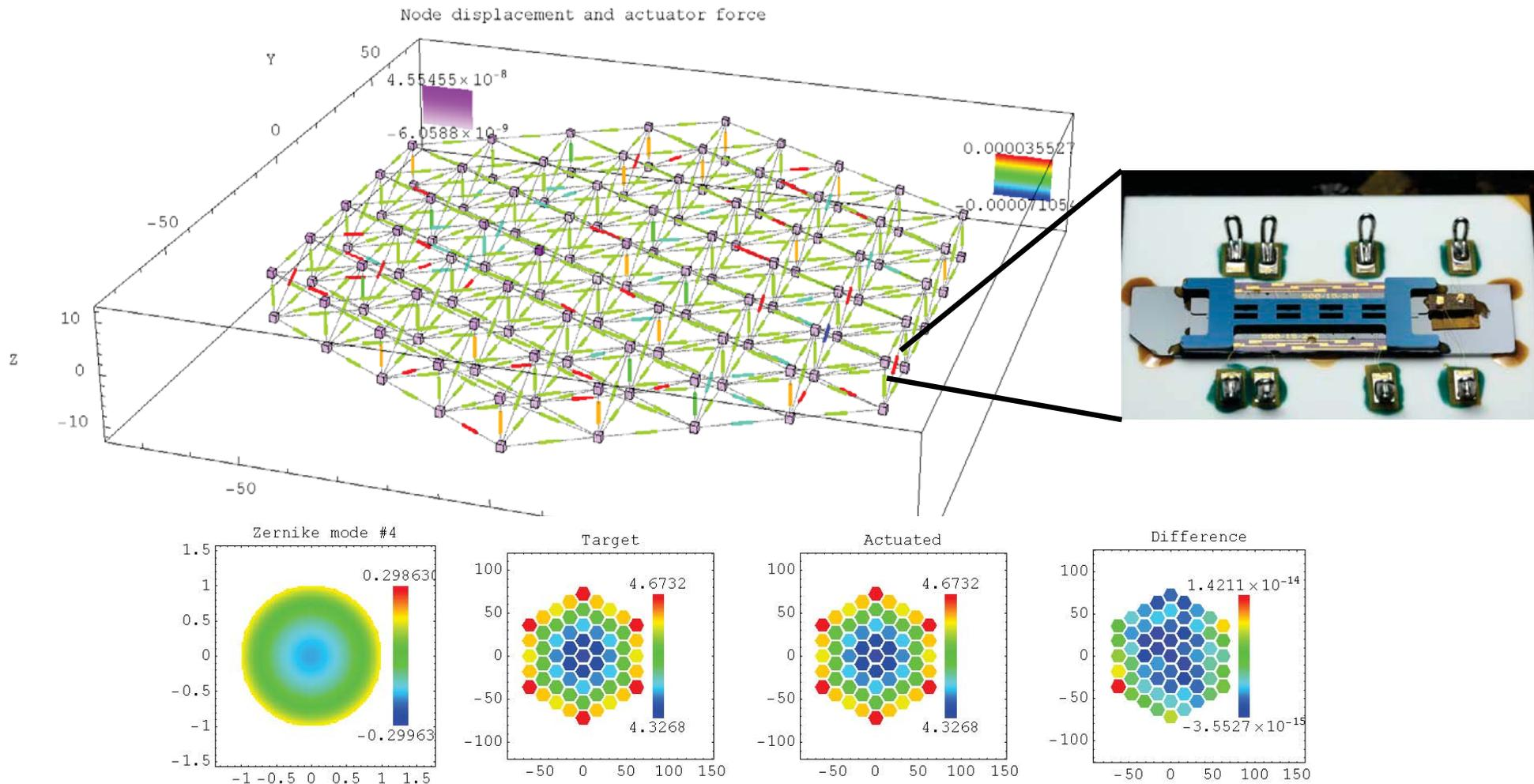
Structure control to the Zernike\* mode 4. Actuator displacement commands were calculated and were subsequently applied, and the structure response to the commands was computed.
