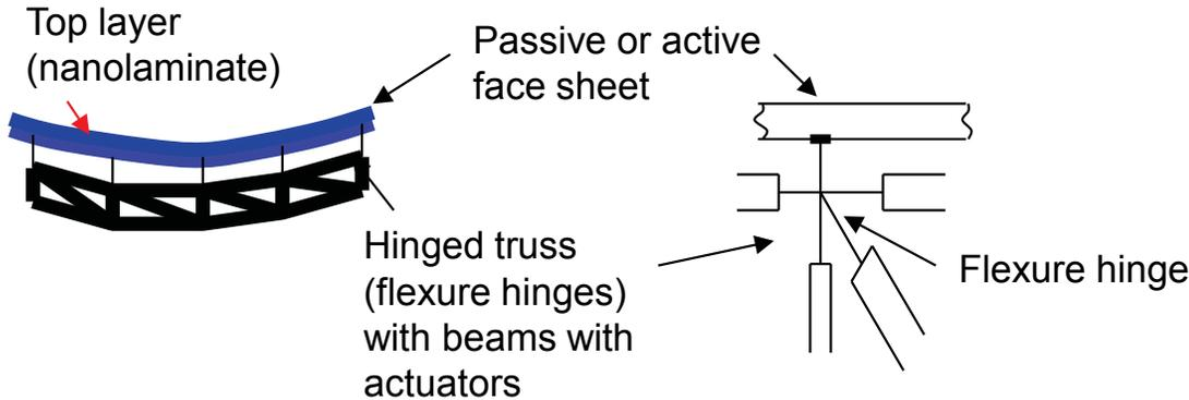
Ultra-large, ultra-lightweight, nanolaminate-based space telescope mirror concept.
