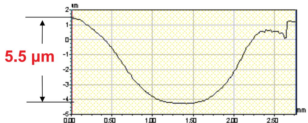
WYKO interferometer image of a PZT unimorph actuator under actuation.
