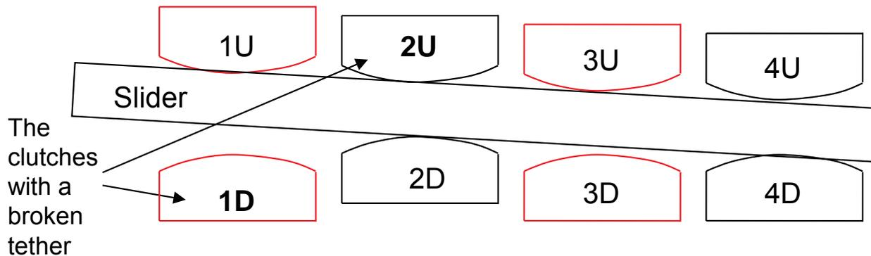
It is more difficult for the clutches to move to the right, because both 1U and 3U are against the movement. In the mean time, there is no resistance against the clutches to move to the left.
