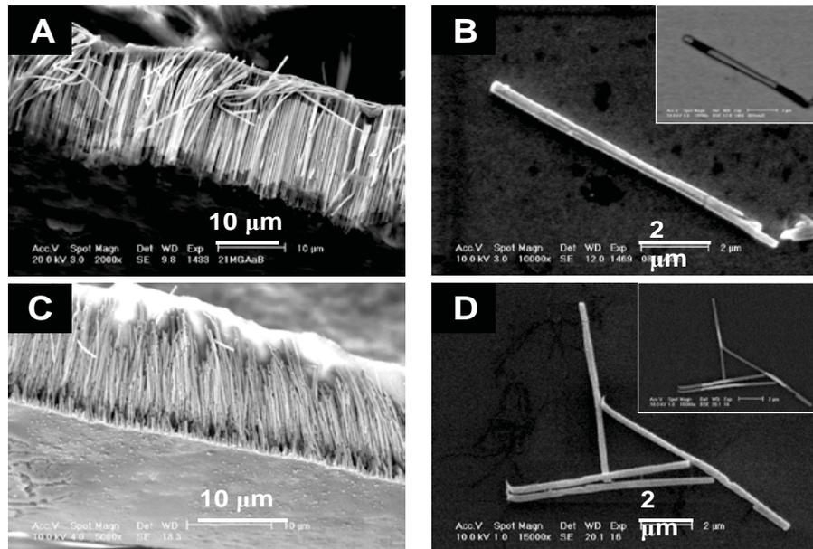
(A) Manganese oxide nanowires, (B) Ni/Au/Ni nanowires, (C) Ni/Bi/Ni nanowires and (D) Ni/Au/Polypyrrole/Au nanowires
