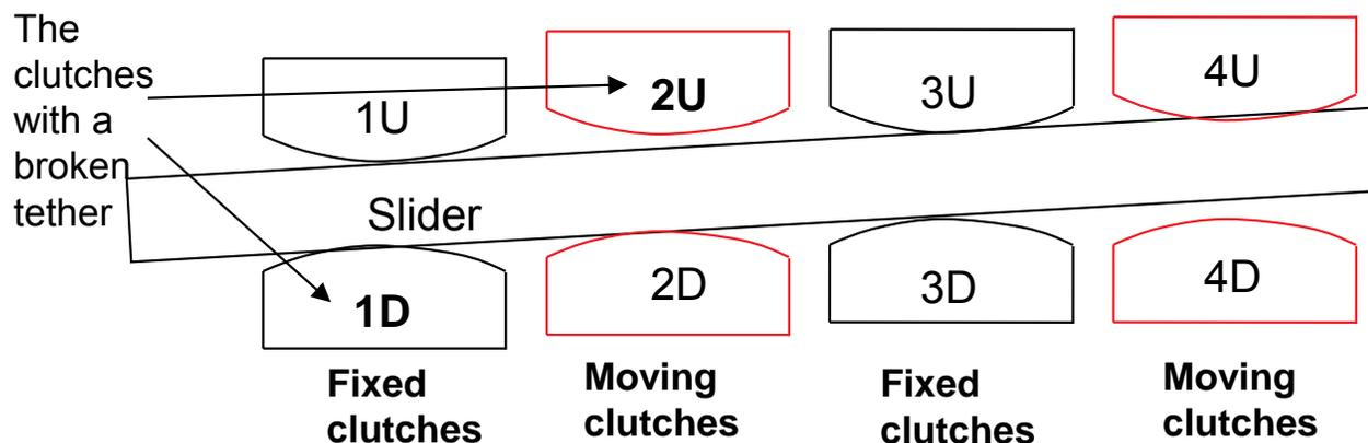
It is about the same for the clutches to move to the right or left, because 2D is against the movement to the right, while 4U is against the movement to the left.
