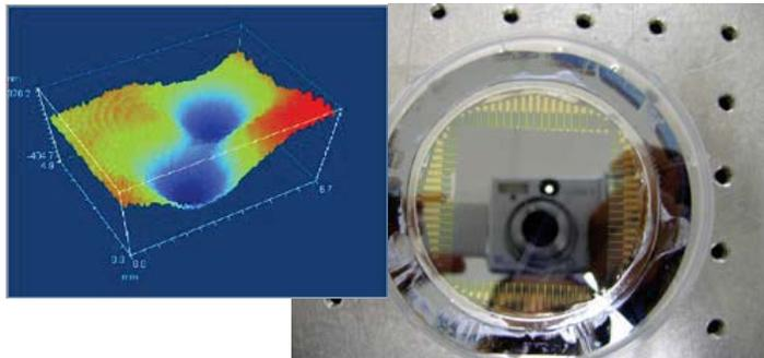
Large-stroke, large-area membrane deformable mirror for ultra-large telescopes
