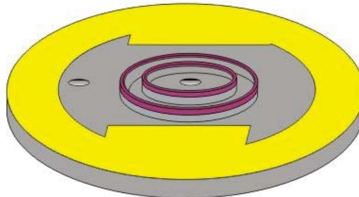
Etching: inlet & outlet holes
