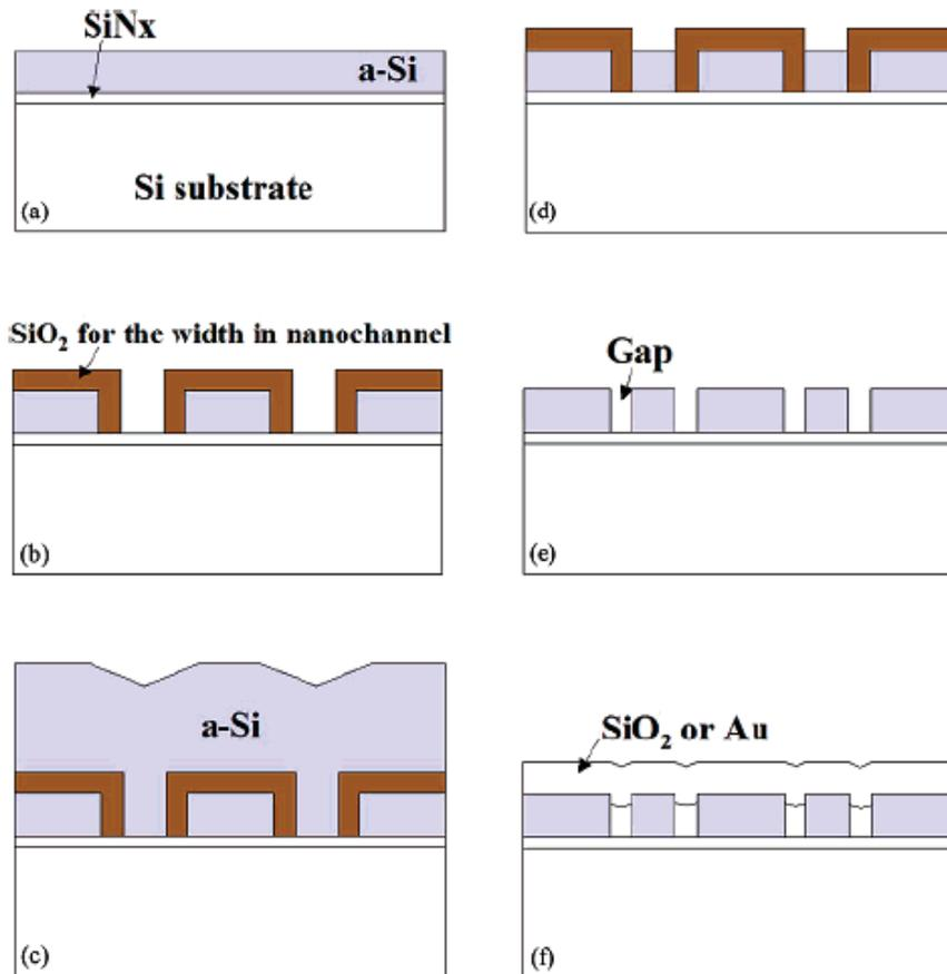
**Figure 1.** Fabrication procedures. (a) SiN<sub>x</sub> and first amorphous Si deposition; (b) RIE and dry O<sub>2</sub> oxidation for the nanometer gap; (c) second amorphous Si deposition; (d) CMP until the gap oxide is exposed. (e) The oxide in the nanometer gap is etched. (f) The Au or oxide layer is used for sealing.
