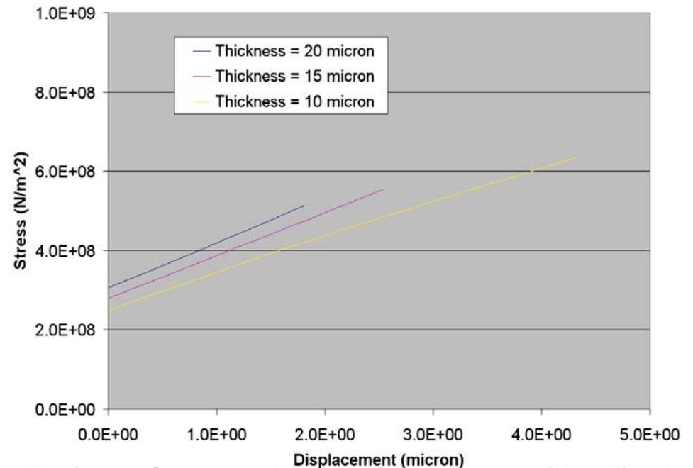
**Maximum-Stress vs. Lateral Displacement with a Fixed Normal Displacement**
