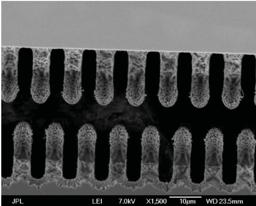
The bottom of the comb is too wide because of insufficient etching.
